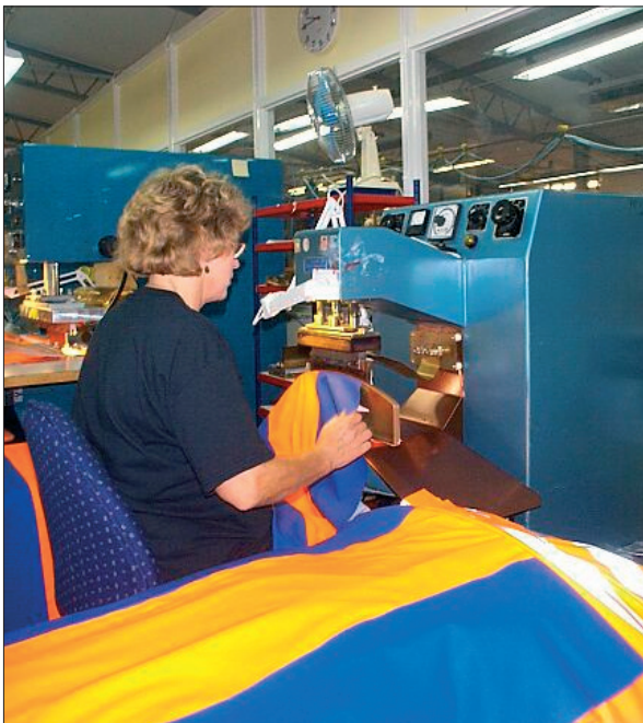
Operating a machine like this the exposure to the head and hands are strong due to the closeness to unshielded electrode.
