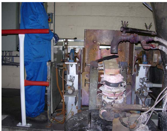
Operator working at a small closed gold melting oven
