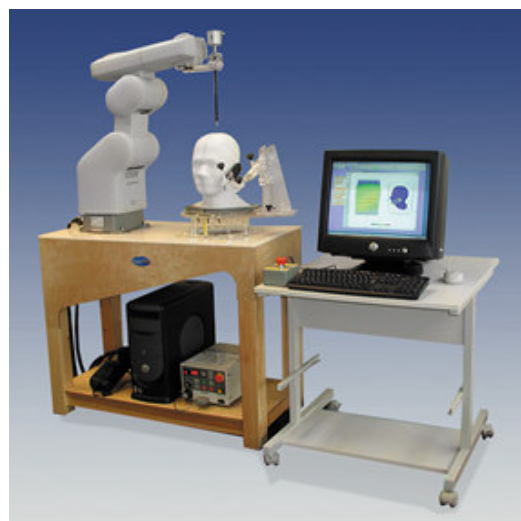
Example of experimental dosimetry set up ( http://www.ets-lindgren.com/ )
